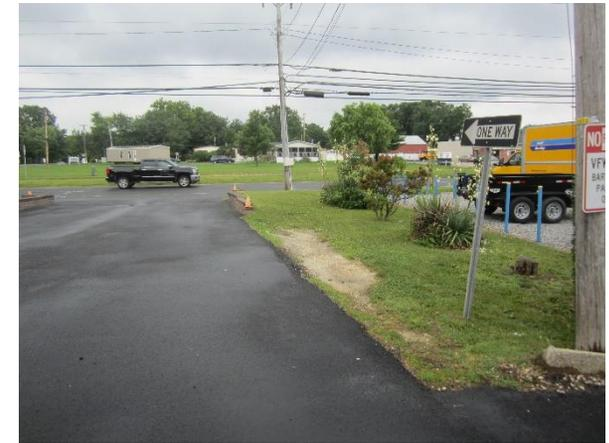
Two sections of parking spaces can be converted to pervious pavement to capture and infiltrate stormwater runoff from the parking lot. A preliminary soil assessment suggests that the soils have suitable drainage characteristics for green infrastructure.
