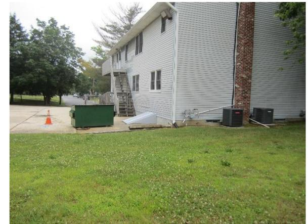
A rain garden can be installed on the southeast side of the building in the turfgrass area pictured above to capture runoff from the impervious roof via downspouts. A preliminary soil assessment suggests that the soils have suitable drainage characteristics for green infrastructure.
