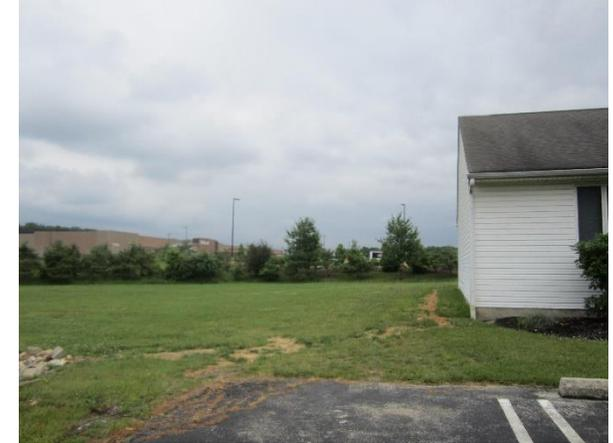
Two rain gardens can be installed on the western and southeastern sides of the building to capture runoff from the roof. A preliminary soil assessment suggests that the soils have suitable drainage characteristics for green infrastructure.
